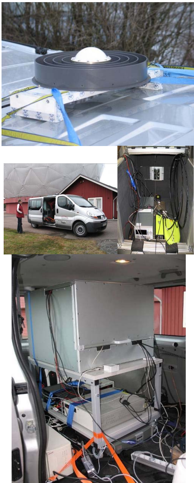
Figure 2. Experimental setup. Top: Dorne-Margolin choke-ring antenna on top of rover. Middle left: The rover at OSO. Middle right: The TIC and the rover GPS carrier-phase receiver inside the box. Bottom: Temperature-stabilised box on top of carry inside rover and transported caesium clock below.
